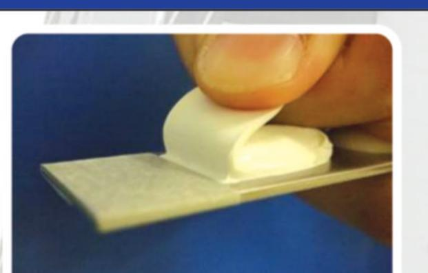
Cohesive failure (MS Polymer)
