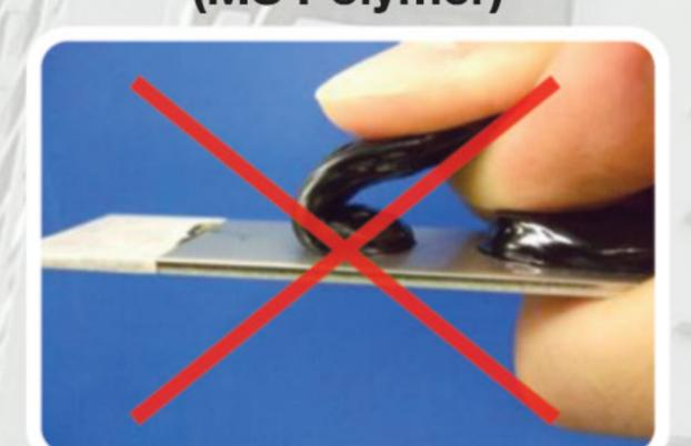
Adhesive failure (Silicone Sealant)
