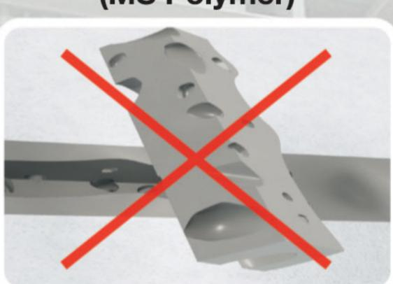
Bubbling (PU Sealant)
