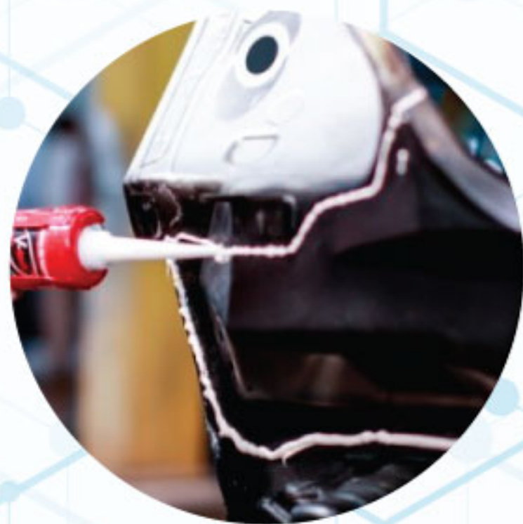
WELDING SEAM SEALING
