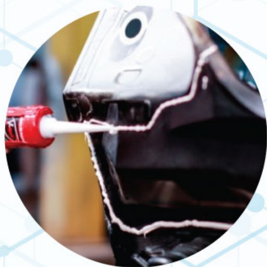
WELDING SEAM SEALING
